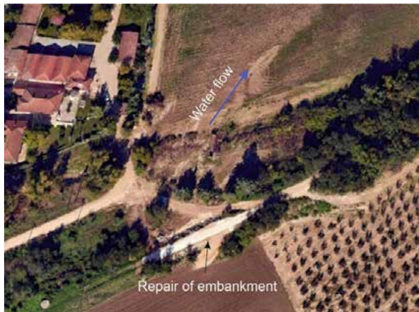
Figure 5. Google Earth scene of the repaired embankment at Alsos locality. The blue arrow shows the flow direction and mud deposition on the cultivated lands. This embankment failure caused by extensive overtopping of the Pineios River.
