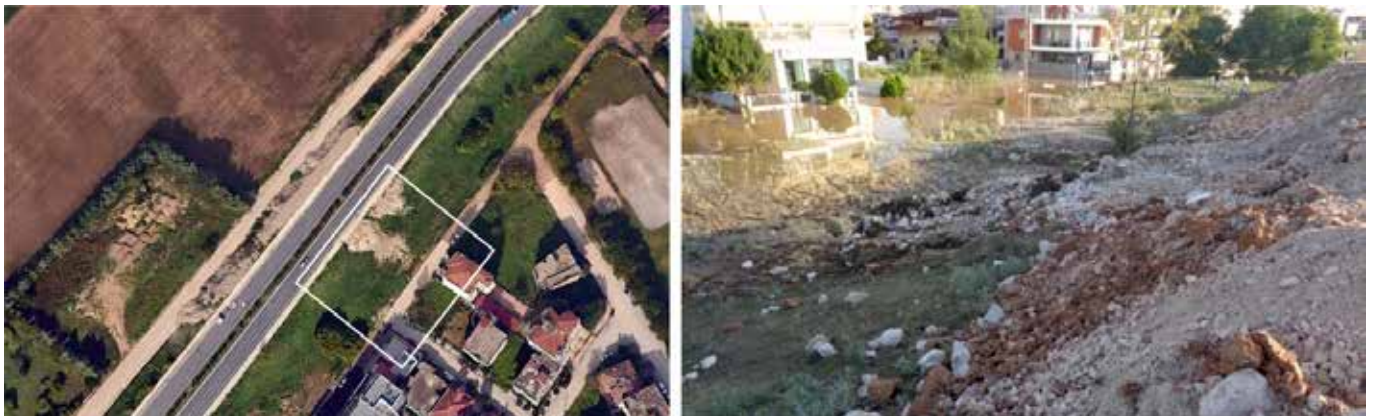
Figure 4. Google Earth scene (left) and field photo (right) of piping failure at locality Stadium just after the Pineios River flooding. The white rectangle in satellite scene show the area of field photo.
