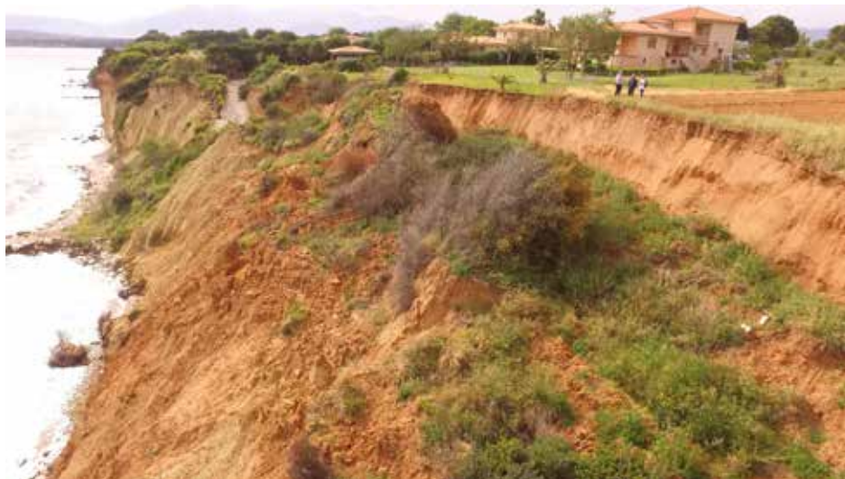
Figure 2. Aerial photograph of the sandstone slope failure occurred in Kalamaki, Western Achaia (UAV campaign, 9/5/2022).
