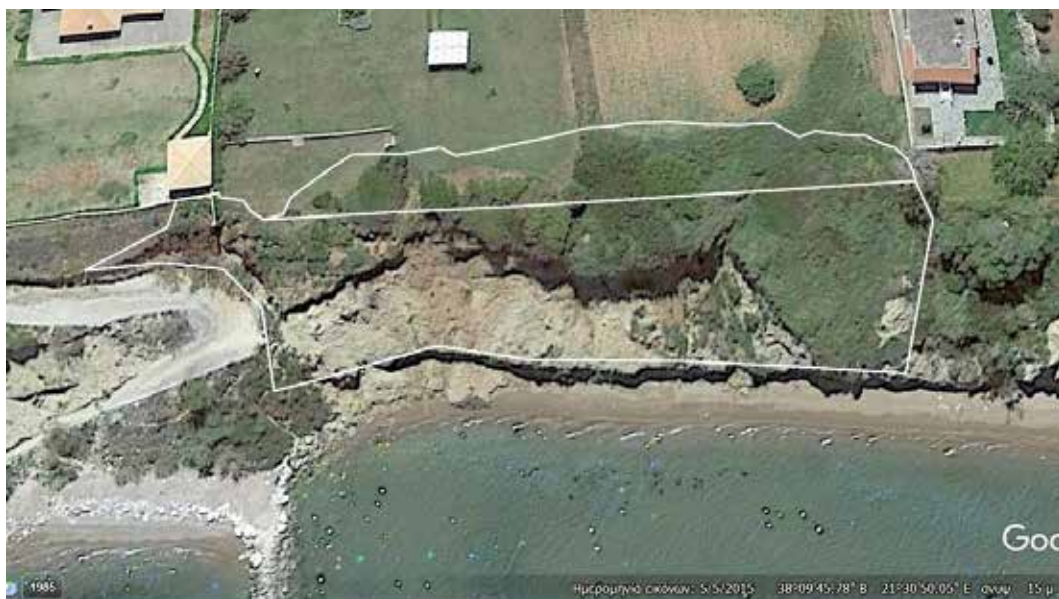
Figure 1. Satellite image of Kalamaki in Western Achaia, Greece (Google Earth 05/2015) with the white line representing the failure area as determined in 9/5/2022.
