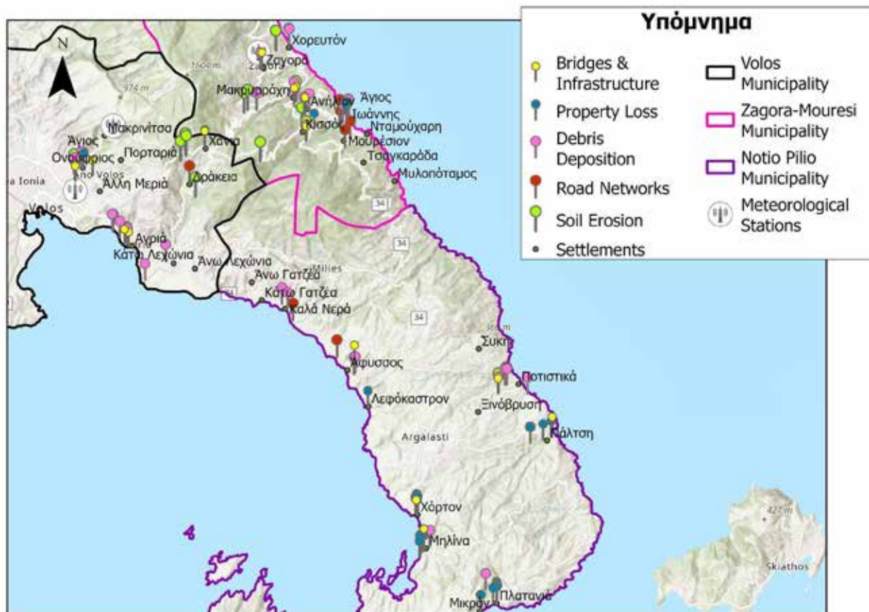
Figure 4. Distribution of types of damages in relation to each municipality of the study area
