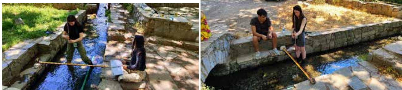
Figure 4. Flow measurements taken with an appropriate flow gauge at the “Kefalari Agios Ioannis” spring on 30-05-2024 (up) and on 14-07-2024 (down).
