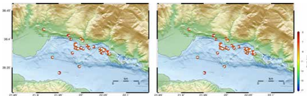
Figure 5. Focal mechanisms of 31 earthquakes during the crisis period, (Left) derived from manually determined FMPs and grid-search over adequate fault plane solutions, (Right) derived with DTM+HASH. The common events presented are those for which the DTM+HASH solutions yielded a quality grade A.
