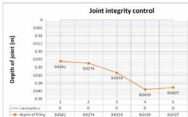
Figure 5. Graph presenting the depth of the open joint; the part of the joint that failed to get properly filled with grout. The graph presents the readings obtained at the joint depicted in Figure 3.b.
