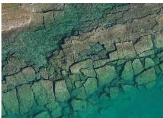
Figure 2. Part of the orthomosaic of the Plaka beach (Drepano, N Argolic Gulf), providing a clear and detailed image of the beachrock formation extending to a depth of -1.20 \pm 0.05 m below mean sea level.
