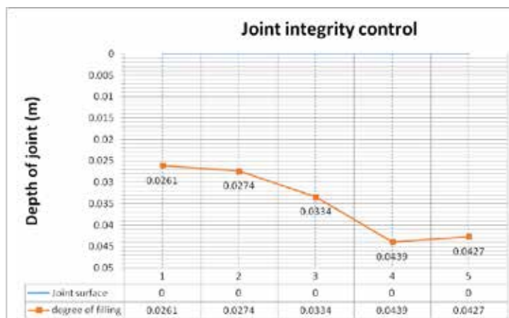
Figure 5. Graph presenting the depth of the open joint; the part of the joint that failed to get properly filled with grout. The graph presents the readings obtained at the joint depicted in Figure 3.b.
