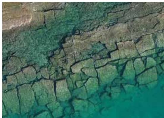
Figure 2. Part of the orthomosaic of the Plaka beach (Drepano, N Argolic Gulf), providing a clear and detailed image of the beachrock formation extending to a depth of -1.20 \pm 0.05 m below mean sea level.
