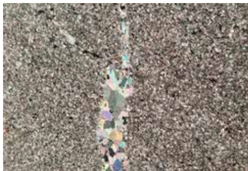
Figure 5. Microstructure in the polarizing microscope of sample 3 (Nicols vertical with magnificence 100x). Presence of sparitic vein in a micritic mass with calcite.
