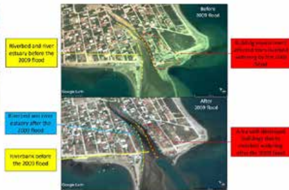
Figure 8. Illustration of the riverbed and estuary morphology of the Lilas River before the 2009 flood (above), as well as the destroyed buildings during the 2009 flood due to the widening of the riverbed (below).
