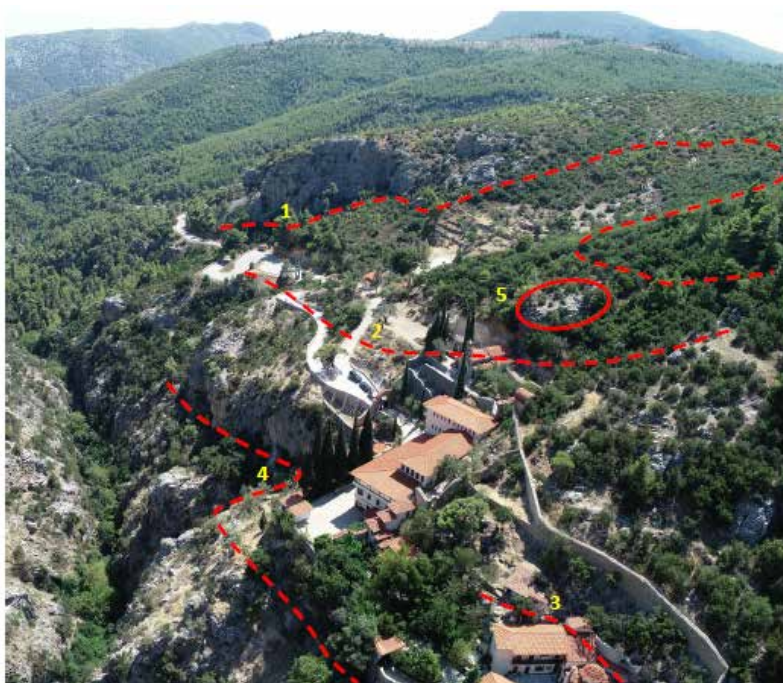
Figure 2. UAV image showing the synthetic depiction of the tectonic contacts at the Holy Monastery of Kleiston. 1: Upper thrust which places the carbonate rocks above the volcanosedimentary rocks. 2: Lower thrust which positions the volcanosedimentary formation upon the carbonate rocks. 3: Upper low-angle fault surface located at the main foundation level of the Monastery. 4: Lower low-angle fault surface situated at lower elevation than the main foundation level of the Monastery. 5: Carbonate fragment.
