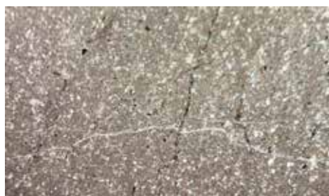
Figure 7. Microstructure in the polarizing microscope of sample 4 (Nicols vertical with magnificence 100x). Homogeneous microstructure with micritic texture.
