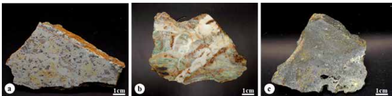
Figure 2. Hand specimen of different types of listvenite (a) Transition rock type (Type I), (b) Carbonate-rich listvenite (Type II), (c) Silica-rich listvenite (Type III) with mineralization
