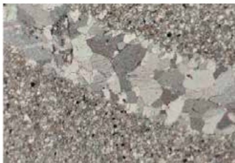
Figure 3. Microstructure in the polarizing microscope of sample 1 (Nicols vertical with magnification 100x). Sparitic vein with isometrical calcite crystals developed in a mainly micritic microstructure.
