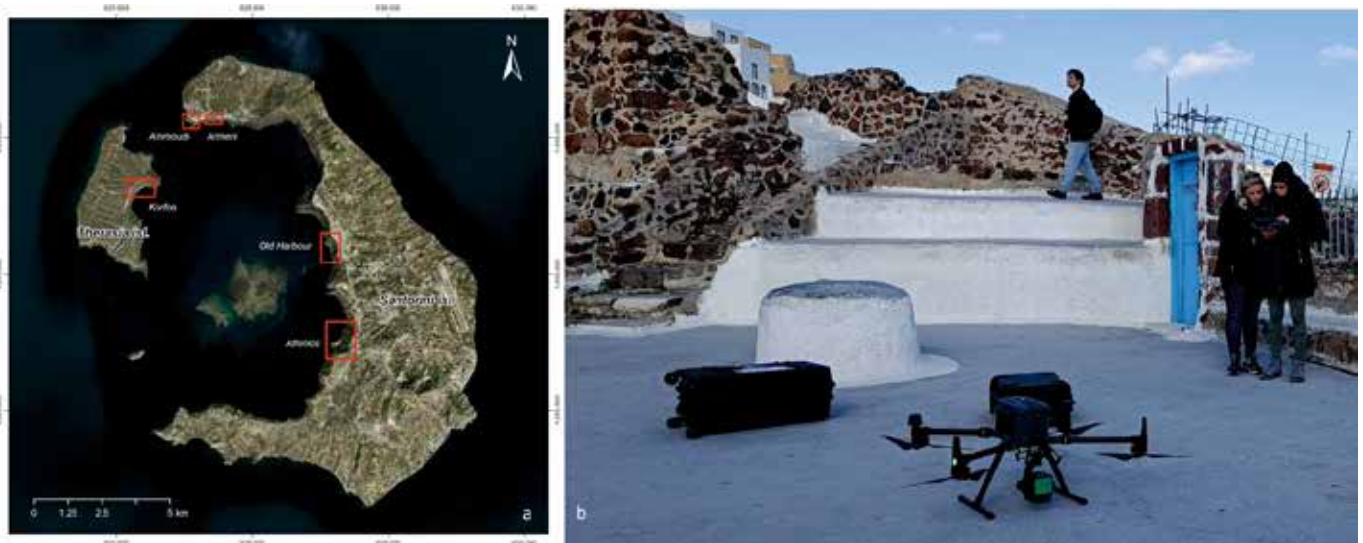
Figure 1. Index map of Thira volcanic complex with the areas of interest marked with red rectangles (a) and the equipment involved with the LiDAR sensor mounted on the UAV (b).
