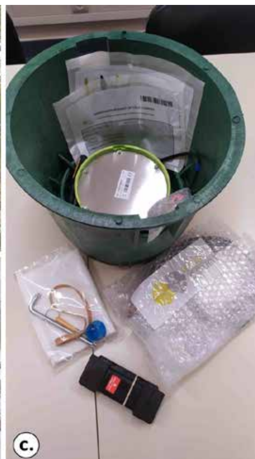
Figure 3. a. Detail of the counting system that was installed at key geosites and geomorphological formations. b. Field work photograph during the installation of the system. c. Detail of the rugged case protecting the logging-transmitting digital apparatus.
